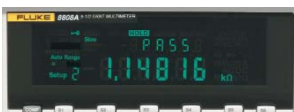
Use setup keys (S1-S6) for fast access to repetitive measurements. Setups can include limit compare mode with pass/fail indicators
